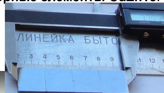
Blanks 19,42 * 19,42 * 5,00 mm to within +/- 0,05 mm (for 256-pix array 40*40 mm (pitch 2,46 mm))
